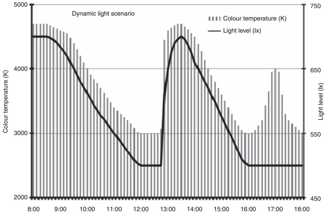
**Figure 1** The dynamic lighting scenario: Illuminance and correlated colour temperature of the lighting plotted against time of day
